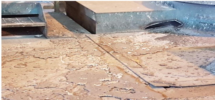
Figure 4. Molten metal leak due to premature lining failure during sintering.
